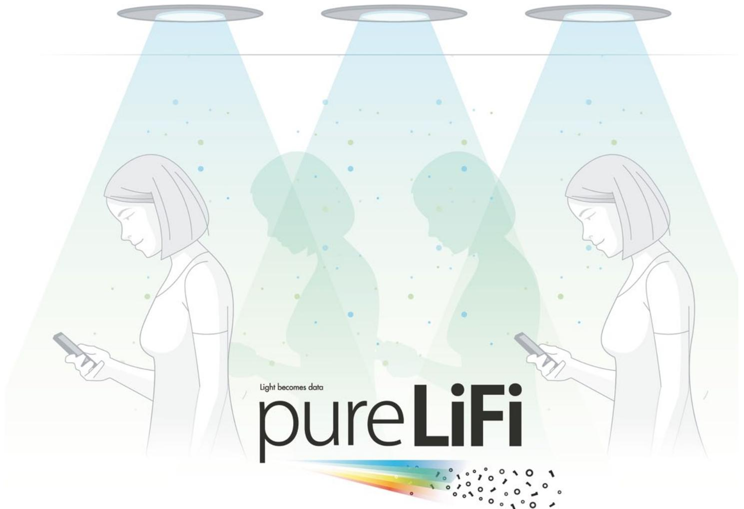
The principle of using light to transmit data is well established, from the TV remote to the lasers that send data down fibre optic cables. However, LiFi enables a fibre-like experience in free space, providing almost unlimited wireless data rates. My group at the University of Edinburgh has shown that it is possible to reach 1 Terabit/second in the foreseeable future without expensive beamsteering technology—which would mean, for example, that a 5 GB video could be downloaded in 0.04 seconds.
